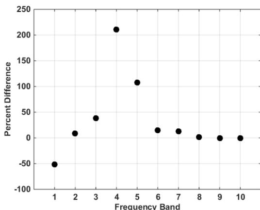
Fig. 9. Percent difference in signal energy magnitude for Bus 1 and Bus 2 ground faults; high Z grounded, 4.7 nF C coupling
