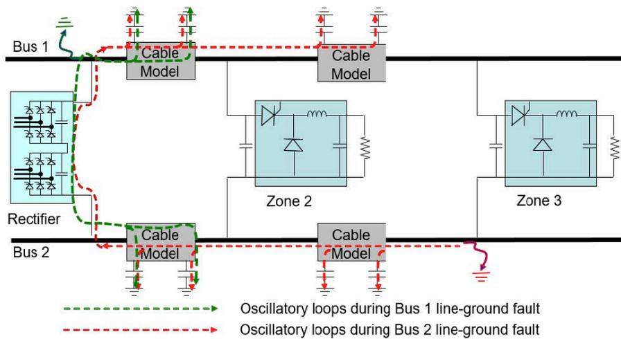
Fig. 3. Characteristic grounding loops within a shipboard distribution system
