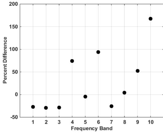
Fig. 11. Percent difference in signal energy magnitude for Bus 1 and Bus 2 ground faults; 470 nF C coupling
