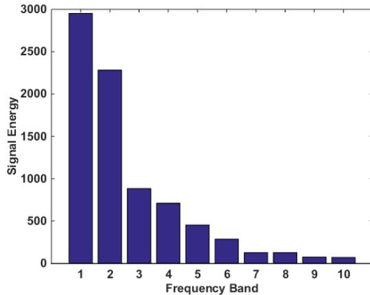
Fig. 5. Wavelet decomposition of noise signal present during a ground fault on positive rail of Bus 1; 4.7 nF C coupling
