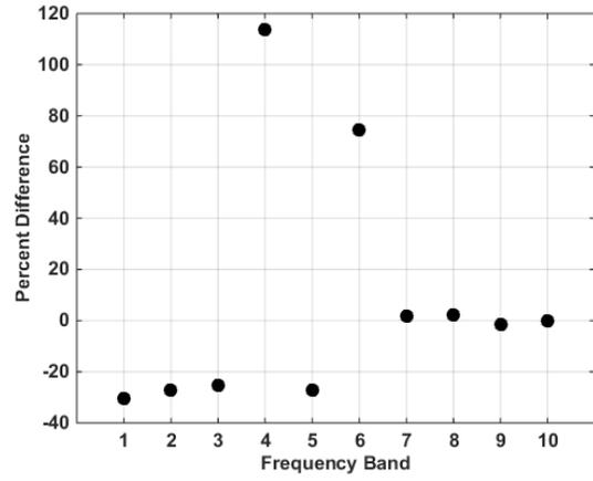
Fig. 13. Percent difference in signal energy magnitude for Bus 1 and Bus 2 ground faults; high Z grounded, 470 nF C coupling
