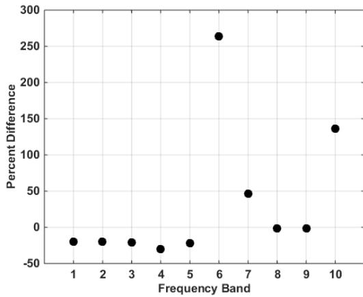
Fig. 12. Percent difference in signal energy magnitude for Bus 1 and Bus 2 ground faults; 4.7 μF C coupling
