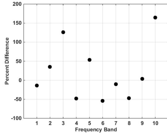
Fig. 7. Percent difference in signal energy magnitude for Bus 1 and Bus 2 ground faults; 4.7 nF C coupling
