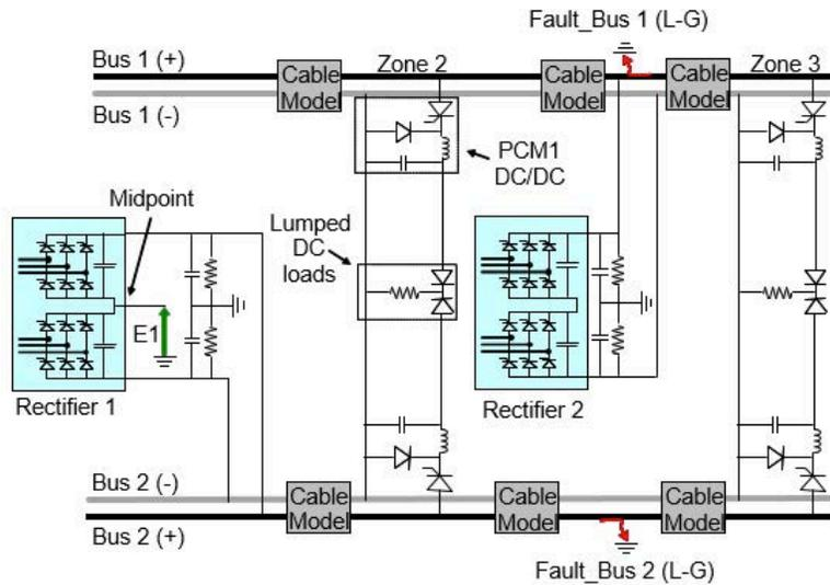
Fig. 4. Diagram of notional two zone MVDC shipboard distribution system EMTDC model used for sensitivity analysis
