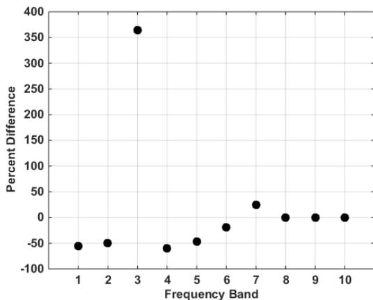
Fig. 10. Percent difference in signal energy magnitude for Bus 1 and Bus 2 ground faults; high Z grounded, 47.0 nF C coupling
