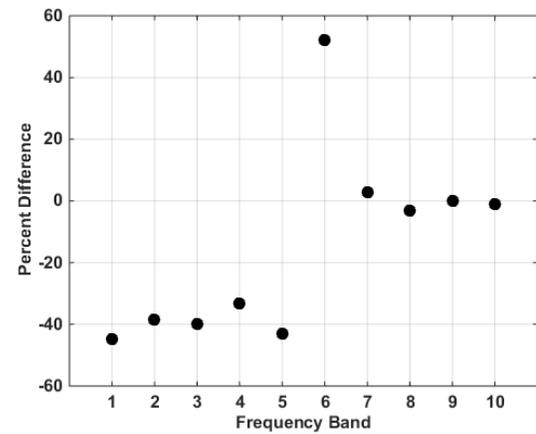
Fig. 14. Percent difference in signal energy magnitude for Bus 1 and Bus 2 ground faults; high Z grounded, 4.7 μF C coupling
