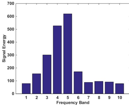
Fig. 6. Wavelet decomposition of noise signal present during a ground fault on positive rail of Bus 1; 4.7 μF C coupling
