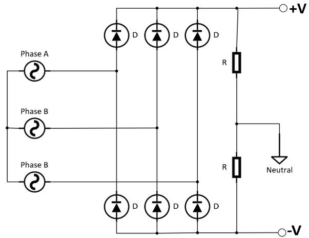
Fig. 2. Resistor Divider Neutral
