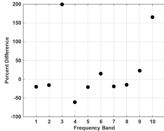
Fig. 8. Percent difference in signal energy magnitude for Bus 1 and Bus 2 ground faults; 47.0 nF C coupling
